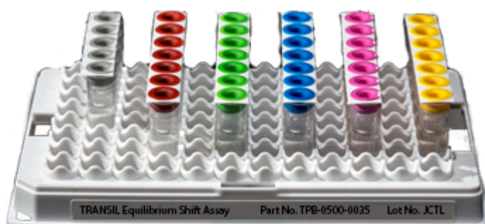
Figure 1: Prefilled tubes supplied with the TRANSIL Equilibrium Shift Assay kit. For each plasma dilution the kit supplies 5 tubes with varying TRANSIL content and 2 reference tubes. For the lowest and highest plasma dilution (i.e. highest plasma concentration), the kit supplies 5 tubes for preparing a 5-point calibration curve.
